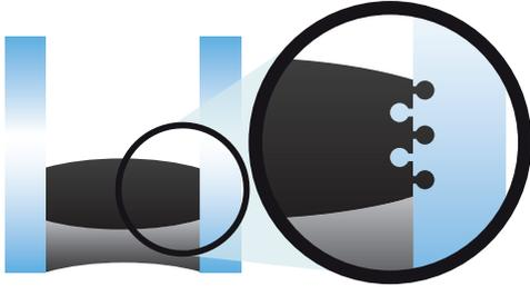
Edge deletion removes coatings, exposing clean glass for a structurally stronger, permanent chemical bond between the **rTPS** spacer and the glass.
