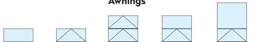
Fixed Lite Awning 2 Lite Awning both operate 2 Lite Awning fixed top 2 Lite Awning 2/3 over 1/3
